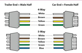
Color coded for conformity to SAE, NMMA, and TMA standards,
