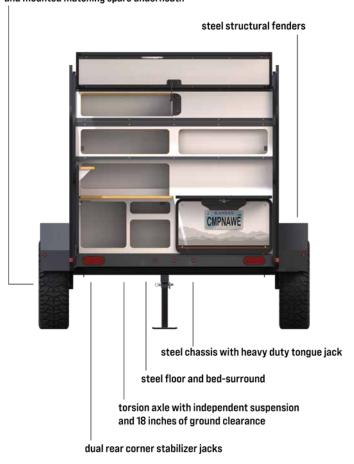
Campinawe's proprietary composite body reduces weight and sits on top of our industry leading heavy duty powder coated steel chassis – all while staying under 2,000 lbs.
